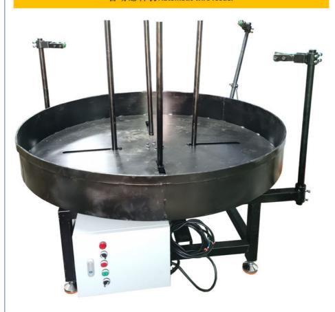
Provide automatic feeding for high-speed machines or automatic machines. It can be used for round wire and flat wire.
