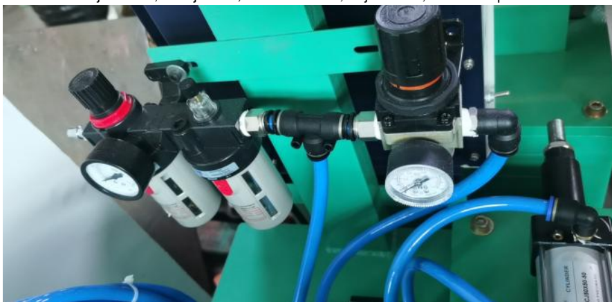
6. Taiwan Yade politely moves the original, air pipe and connector. Independent two-piece, pressure reducing valve, convenient adjustment, oil injection, water filtration, adjustment, more independent.
